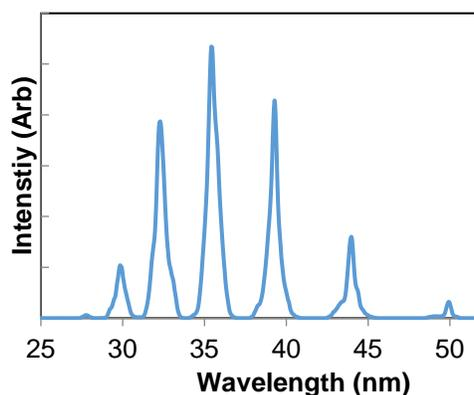
Figure 4 shows the main components used in this successful HHG demonstration. The HHG was analyzed using an EUV imaging spectrometer followed by a EUV CCD array detector. When argon is used as the fill gas, the output consists of several harmonics centered in the “near-EUV” at 35 nm. When helium is used, the output is centered at 13.5 nm in the deep UV. Alternatively, the
