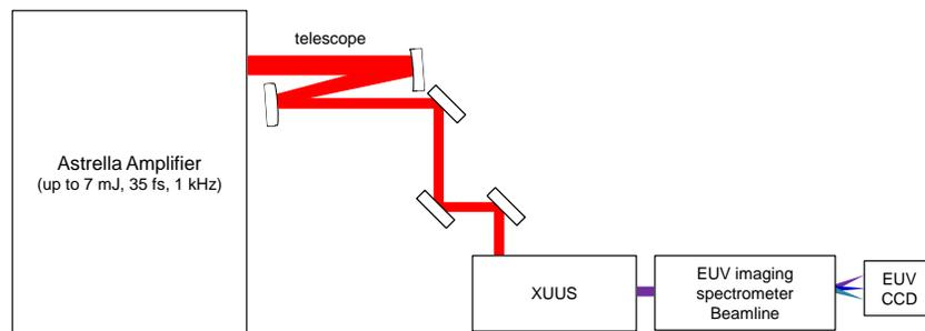
**Figure 4:** Schematic illustration of the setup used to generate EUV pulses. Inset shows the recorded spectrum of the EUV pulses when the HHG gas is helium with an optimized input pulse energy of 6m. The spectral bandwidth (FWHM) of the different harmonics is approx. 0.75 nm.
