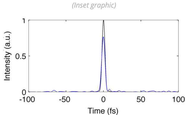
This approach takes advantage of the spectral broadening caused by self-phase modulation (SPM) in a hollow fiber containing a noble gas. The fiber acts as a dielectric waveguide, confining the beam and allowing for a long interaction length at a high intensity. This established approach is proven to allow the generation of high-power (up to 5 mJ), few-cycle laser pulses at kHz repetition rates.
