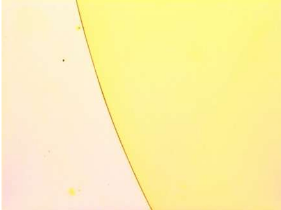
Figure 3. A CO laser with only 9W of output power produced this clean, curved cut (6 mm radius circle) in thin glass (50 \mu\text{m} thick) at a feed rate of 140 mm /sec.
