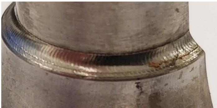
Figure 2: A 1 mm LBW (laser beam weld) fillet weld on a funnel using 308L filler metal. This is a smaller weld joint compared to GTAW with essentially no heat affected zone, no discoloration, and no distortion.
