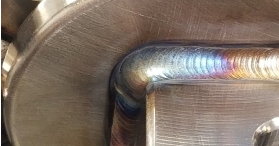
Figure 1: A 0.125" GTAW fillet weld using ER630 filler metal on an implant holder showing some discoloration due to the applied heat. However, GTAW is used here because these parts tend to be thicker and therefore require a deeper penetration weld.
