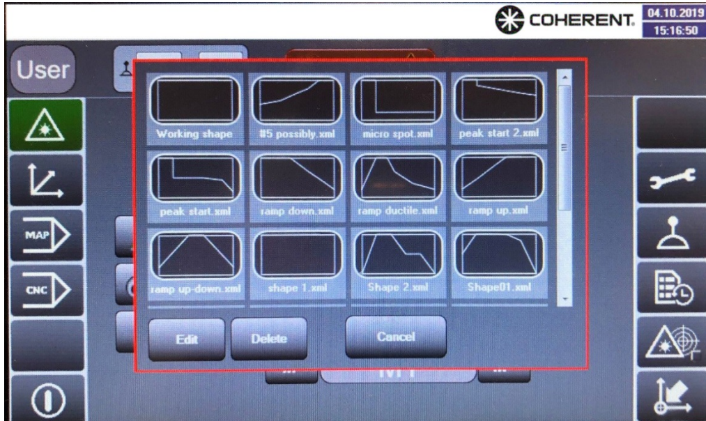
Figure 4: The manual laser welding system Select from Coherent allows the adjustment of the laser pulse shape to optimize the welding results either with pre-programmed or newly programmed pulse shapes.
