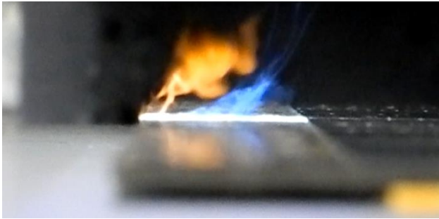
Figure 2: Plasma clouds during 308 nm cleaning of CFRP part
