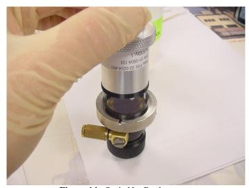
Figure 14. Optic Nut Replacement
