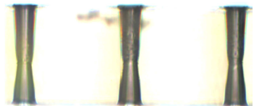
Fig. 5. Side view of through via holes in 100 μm glass obtained with an equal number of pulses from both sides.
