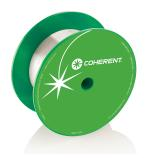
Coherent's Cladding Mode Free (CMF) fiber is designed to allow more uniform grating-writing in WDM applications. CMF virtually eliminates all cladding modes allowing tighter channel spacing for high speed communications. Cladding Mode Free fiber is mode-matched to SMF-28TM for telecommunication system use. The polyimide coated CMF fiber is ideally suited for use in a WDM distributed sensing networks operating in high temperature and harsh environments.
