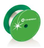
Coherent's specialty multi-mode fibers are ideal for a variety of diverse applications. They are capable of withstanding extreme environments and large temperature swings. Features include step index and graded index configurations, numerical apertures from 0.06 to 0.45 and core sizes from 10 µm to 700 µm. All fibers are available with a high temperature acrylate, silicone, or polyimide coating.
