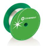
Coherent's specialty multimode step-index fibers are designed for compatibility with the majority of fiber-coupled, bar and stack diode-laser packages and support the diode laser power delivery market. These power delivery fibers are available in 400/440 and 400/480 core/clad ratios in low and high NA versions. The 400/480 has a low refractive index fluoroacrylate coating for added power confinement. Other fiber diameters are available upon request.
